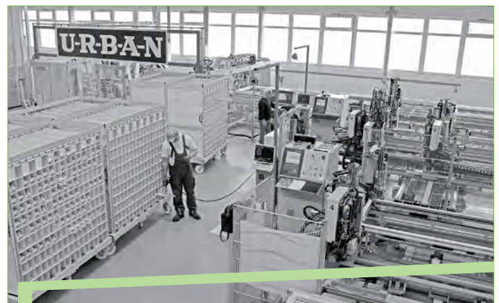
Welding and cleaning line by Urban at Arndt Fenstertechnik
