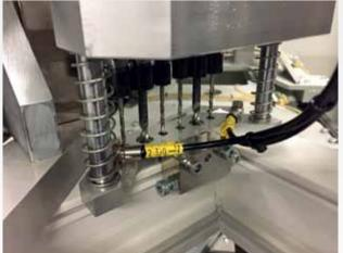
Nothing left to be desired: Drilling unit for cross corner brackets (ESB) by Urban.
